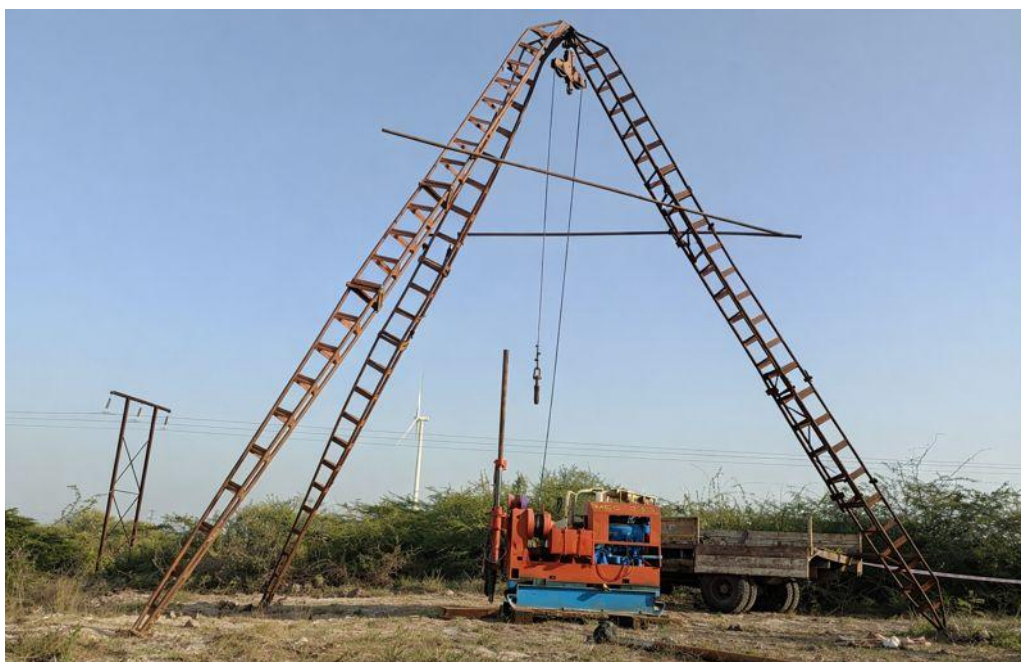
Photograph No.13.1: RD60 drill Rig used for drilling operations
