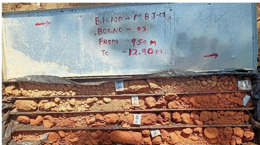
Photograph No.7.7: Core Photograph of MBJ-01 showing Clayey Bauxite intercepted between 07.50 to 13.50m
