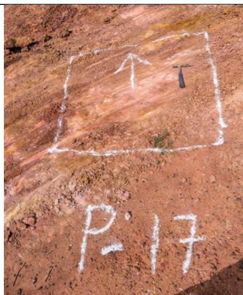
Demarcating the Dimension of Pit
