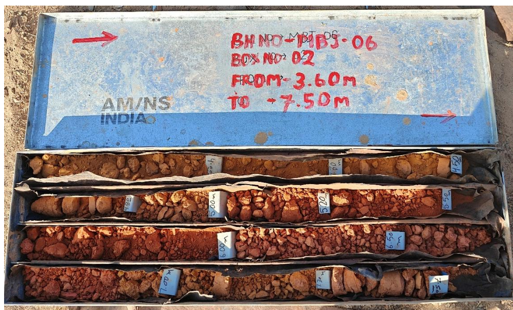
Photograph No.13.4: Drilled core by dry drilling
