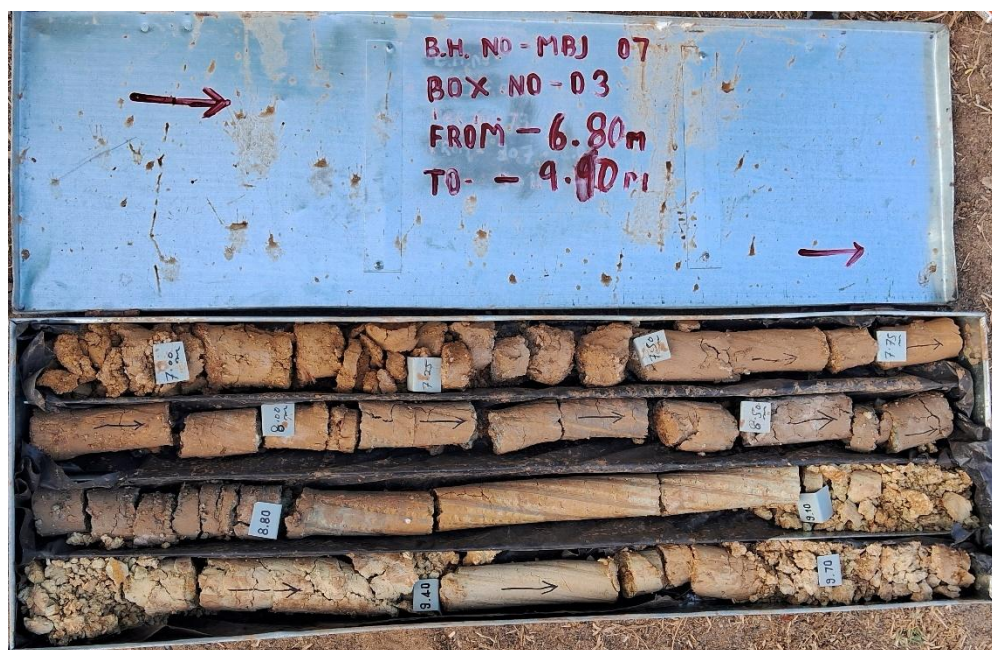
Photograph No.7.8: Core Photograph of MBI-07 showing Lithomargic Clay intercepted between 8.80 to 11.00m
