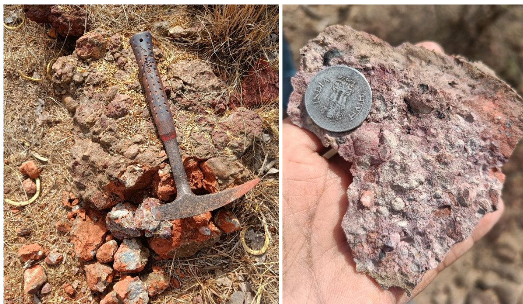
Photograph no 7.5: Conglomeratic and pisolitic Type of Pisolitic Bauxit
